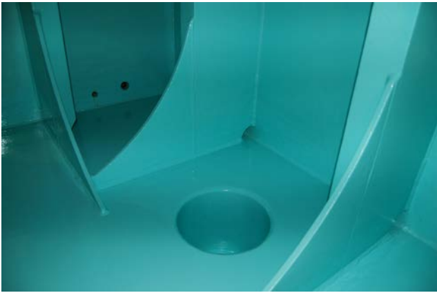
Figure 5.4: This tank has a drain well, and the stiffeners are placed vertically, with drain cavities against the tank floor. Consequently the tank is easy to drain (Photo: Eyvind Andersen)
