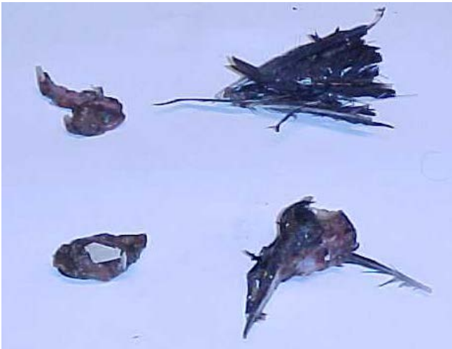
Figure 5.6: The remains of a bird collected from offshore potable water tanks. The bird entered via the bunkering hose, got stuck in a valve, and spread to all the water tanks as it gradually decomposed (Photo: Anonymous in agreement with the company)
