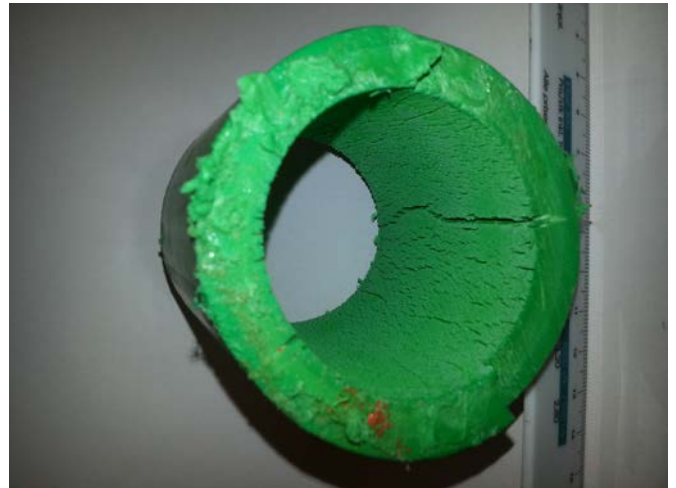
Figure 9.20: Hot water pipe damaged because of lacking expansion tank and too high pressure and temperature in the hot water system (Photo: Johan Ljungqvist)
