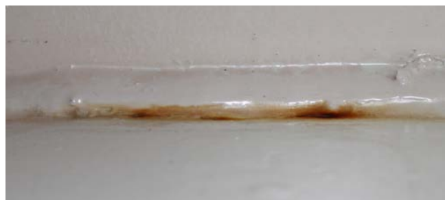
Figure 9.8: Insufficient washing of salts in welding seam before painting has resulted in corrosion (Photo: Bjørn Løfsgaard)
