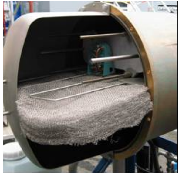
Figure 6.5: Shows the inside of an evaporator. The net prevents seawater drops from passing on to the distillate (Photo: Bjørn Løfsgaard)
