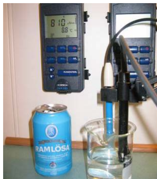
Figure 4.9: Some natural mineral water has very high sodium content, as shown by the conductivity meter (Photo: Eyvind Andersen)
