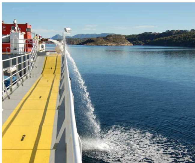
Figure 7.8: Dumping of potable water from tank. Dump “old” water prior to bunkering. This applies to both supply vessels and offshore units (Photo: Eyvind Andersen)
